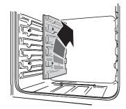
Each side of the oven is fixed with four fixing screws. You don't have to remove the screws to remove the oven linings. Lift each side panel upwards and they will slide off the screws. Then pull them forwards.
